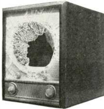
Front view of set damaged by implosion.
