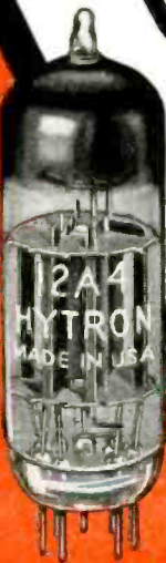
NEW 12A4 → High-efficiency, medium-mu, 9-pin miniature triode. Used as vertical amplifier, class C oscillator, or low-distortion audio output amplifier in push-pull.
